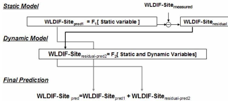
Figure 3. Schematic showing the two-stage model approach to making final water-level difference for a particular site (WLDIF-Site).
