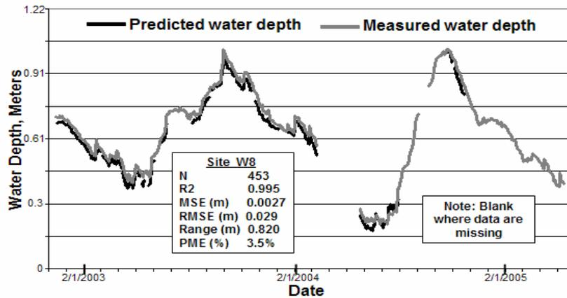
Figure 5. Plot showing measured (light trace) and predicted (dark trace) water depths for Site W8. Predictions are not continuous due to missing data for one or more of the index stations.
