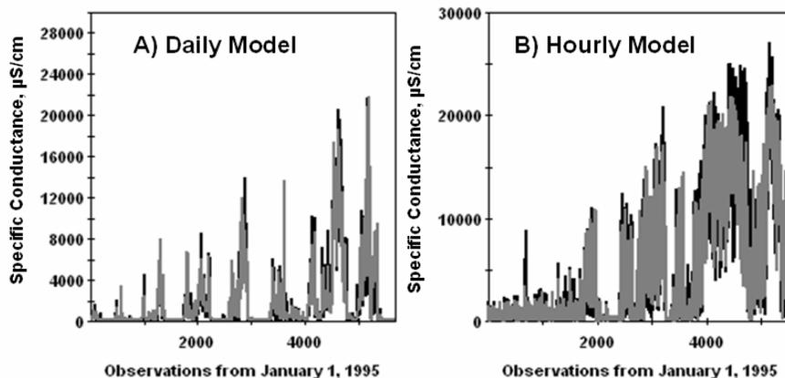
Figure 5. Graphs showing measured (black trace) and predicted (gray trace) specific conductance for Hagley Landing (Station 02110815). Results for the daily model are shown on the left (A) and the hourly model on the right (B).
