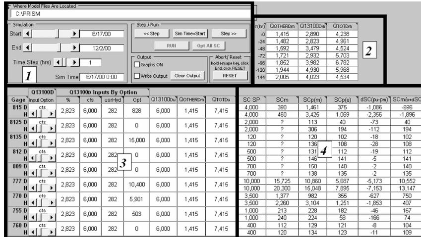
Figure 6. Graphical User Control Panel from Pee Dee River DSS - (1) simulation start/end/step; (2) input streamflow values and 1- to 7-day time delays; (3) user option for modified flows and their inputs; and (4) specific conductance values – measured, predicted, user defined, and impact.
