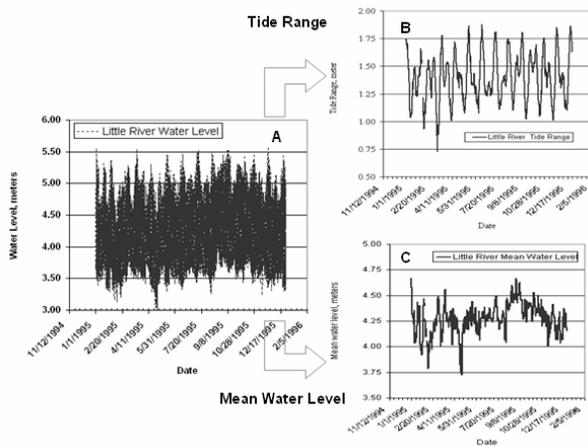
Figure 2. Tidal water-level signal (A), decomposition into a periodic signal of tide range (B), and a chaotic signal of mean water level (C).
